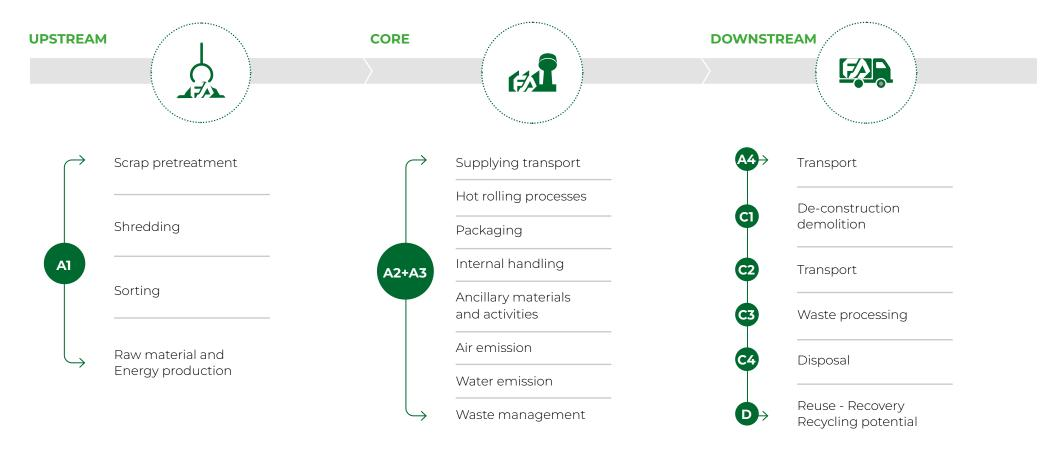
Broad scheme of cold rolled steel production, in which the main activities included in the system boundaries are listed and divided in the three subsystems: UPSTREAM Process, CORE Module and DOWNSTREAM Process
