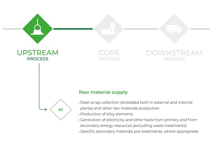
Broad scheme of hot rolled steel production, in which the main activities included in the system boundaries are listed and divided in the three subsystems: **UPSTREAM Process**, **CORE Module** and **DOWNSTREAM Process**.
